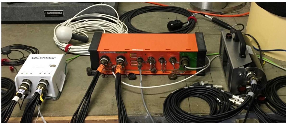
Figure 4 Form Factor Comparison of the Digitizers
