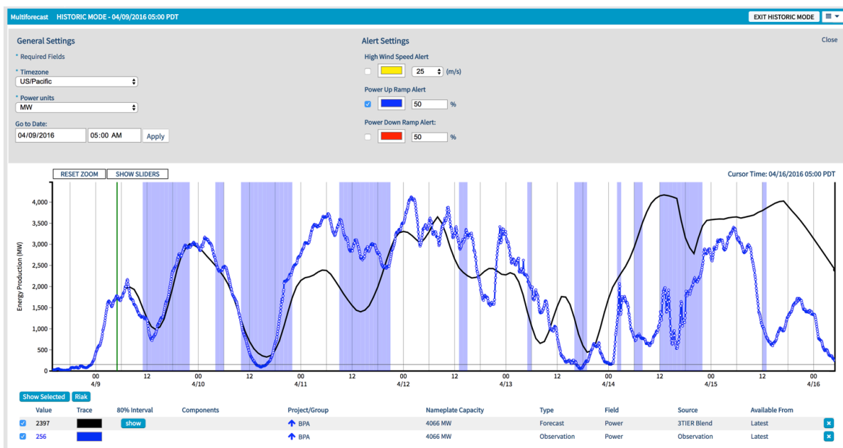
Figure 69. Screenshot of the prototype DST utilizing Vaisala's existing Multi-Forecast Tool with new alert types enabled. The tool is set to Historic Mode displaying the latest hourly-resolution forecast from April 9, 2016 at 05:00 PDT for the BPA fleet aggregate wind power (black curve) along with the corresponding 5-minutely power observations (blue dots). Only alerts for generic up-ramp events are activated and shown in the forecast time-series as blue color-shaded regions where the probability exceeds the 50% critical threshold. A corresponding blue up-arrow icon is shown in the legend for the affected project (BPA).
