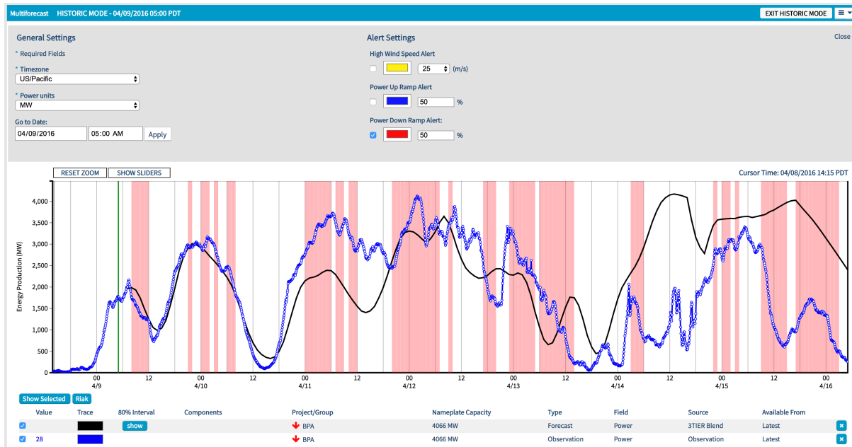
Figure 70. As in Figure 69, except with only generic down-ramp event alerts activated. The alerted hours are shown in the forecast time-series as red color-shaded regions where the probability exceeds the 50% critical threshold. A corresponding red down-arrow icon is shown in the legend for the affected project (BPA).
