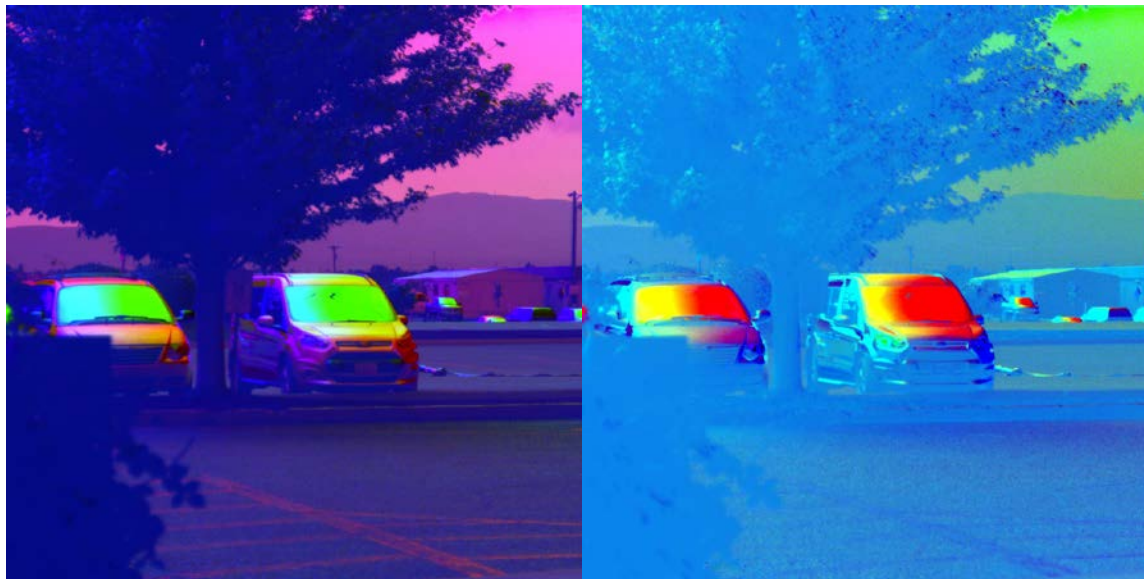
Figure 2.3. Data from the images in Figure 2.2 combined as false colors. Left - S0=red, S1=green and S2 = blue; Right – S1=red, S2=green, S3=blue. Windshield reflections exhibit the most polarization effect and are strongly associated with S1, as expected.
