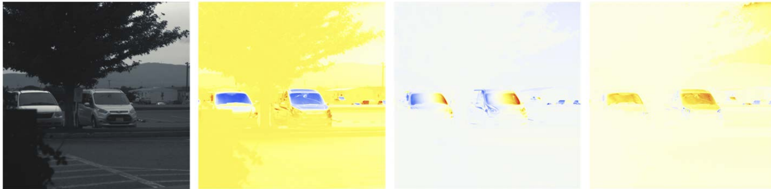
Figure 2.2. (From left to right) S0, S1, S2, and S3 Polarization Images of the Same Scene. S1 is strongly associated with reflections off the windshields and car hoods while S2 is dominant on the slightly curved windshield edges.
