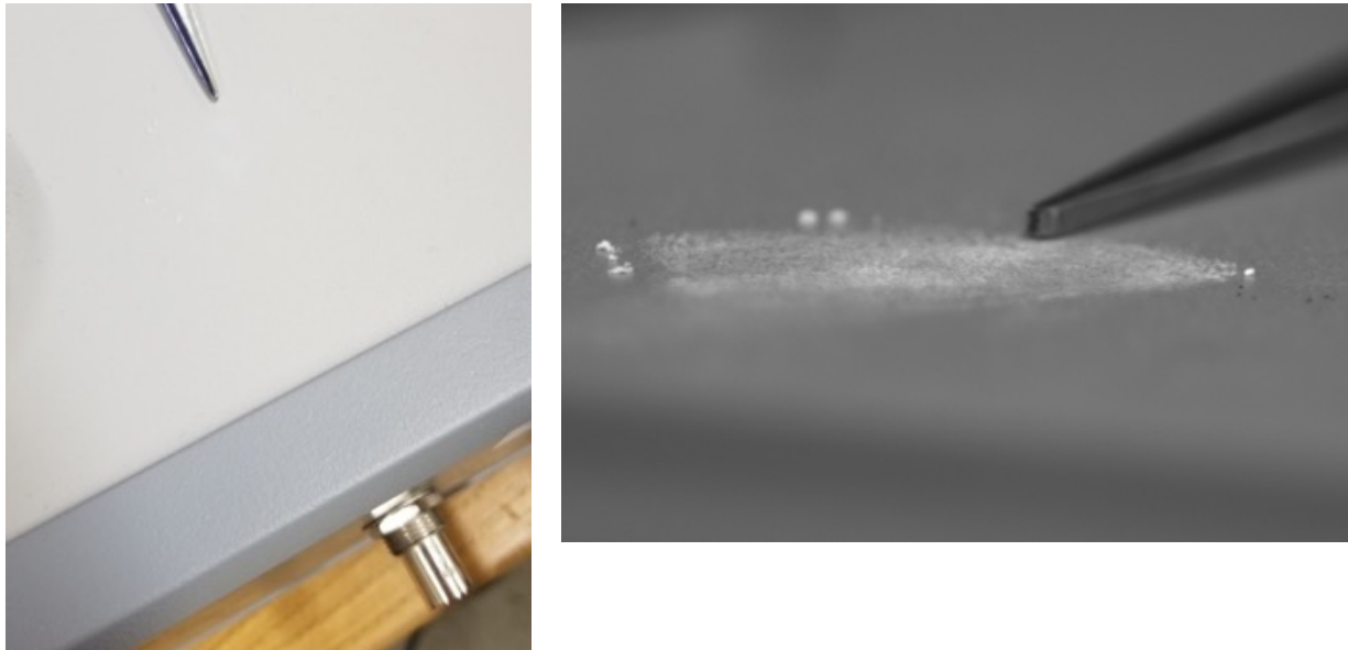
Figure 3.1. Neodymium Oxide on a Painted Electrical Box. The powder was rubbed into the textured paint in the area just below the metal pointer. The left image is a regular color photograph. On the right is a polarized image of the same area.
