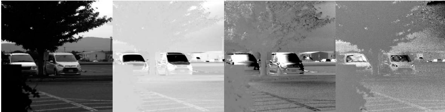
Figure 2.4. Principle Components Analysis of Salsa Images using ENVI Software Showing Greater Detail than the Pure Stokes Images.
