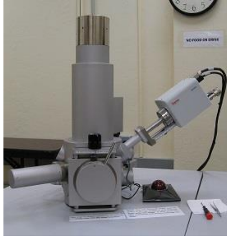
Fig. 5.5. Tescan Vega 2 SEM (a) and Zeiss Ultra plus FESEM (b) instruments used for sample characterization.
