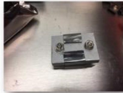
Fig. 5.4. Diffusion couple fixed in a molybdenum-jig inside a glovebox.
