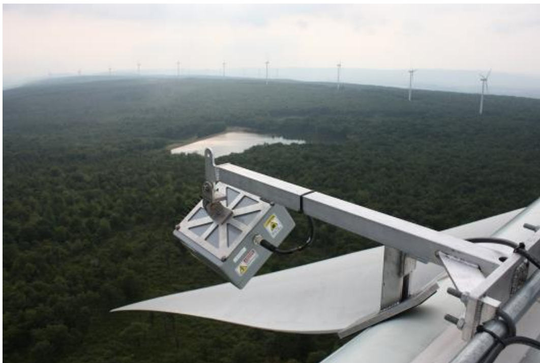
Figure 2. Photograph of the Deaton UAD secured to the wind turbine by a cantilevered arm.
