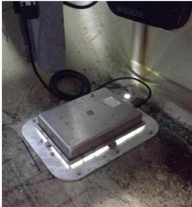
Figure 9. Photograph of a prototype UAD installed on the floor of the nacelle.
