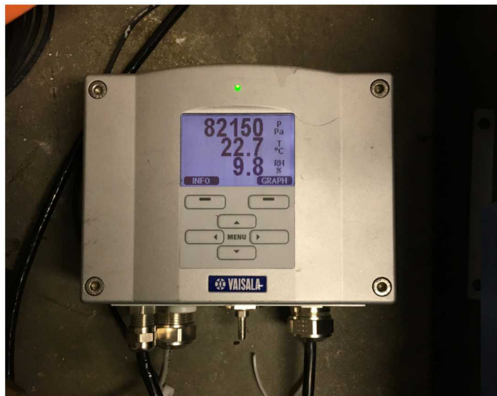
Figure 5 Vaisala temperature monitor within the FACT bunker
