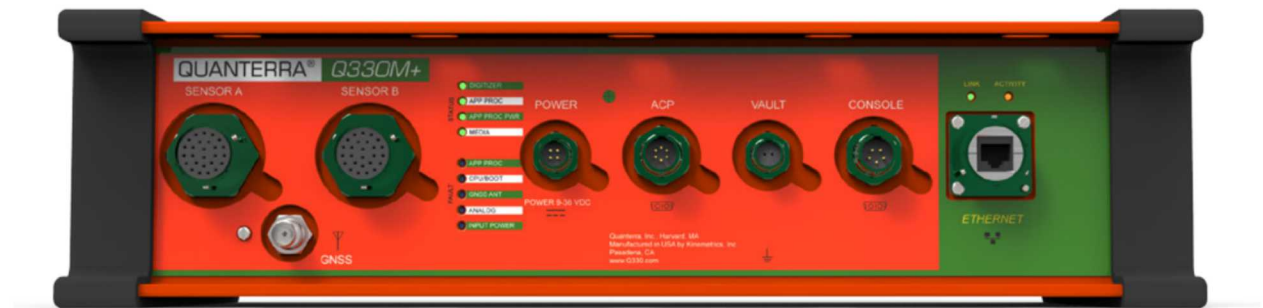
Figure 1 Quanterra Q330M+ digitizer. Photo courtesy of Kinemetrics, Inc.
