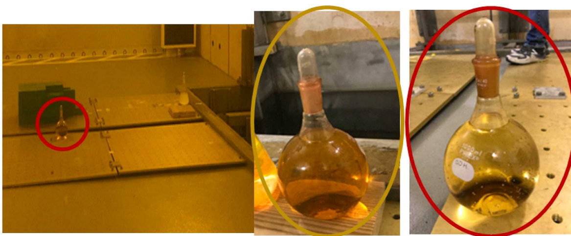
Figure 9. Images of the R6G sample #1 during testing (A), after 5 min irradiation (B), and after 360 min irradiation (C).
