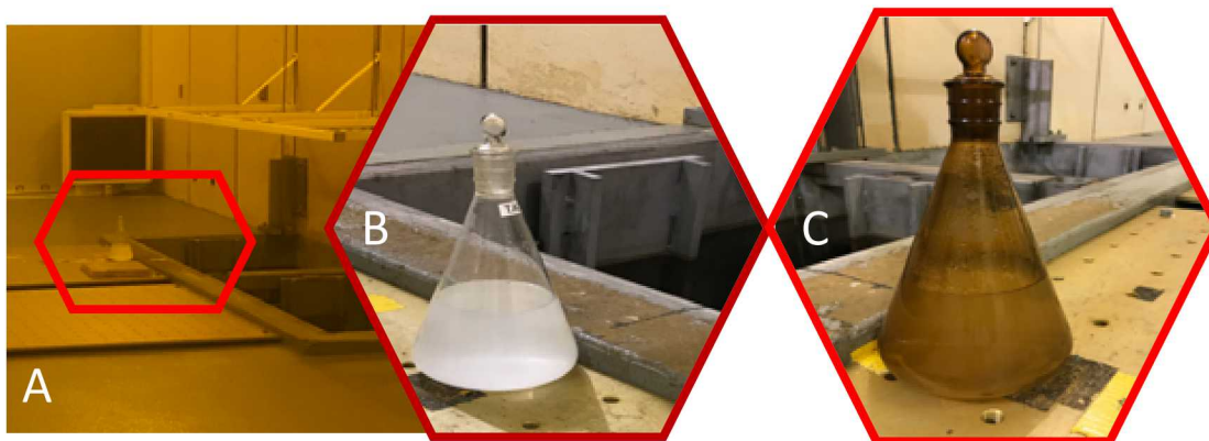
Figure 11. Images of the TAD sample (A) during testing, (B) before irradiation, and (C) after 360 min irradiation.
