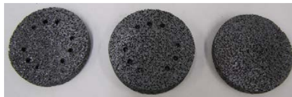
(b) Machined graphite foam disks
