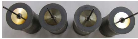
(e) Completed corrosion test modules
