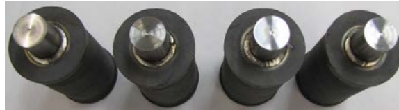
(f) Capped corrosion test modules
