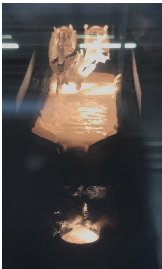
Fig. 3.4. Photograph during CHM showing molten metal in crucible and hearth, with partially melted Ti-Nb feedstock tubes
