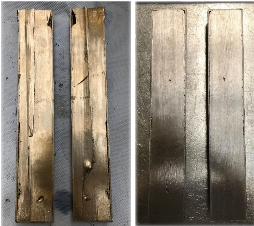
Fig. 2.6. Photographs of cross-sectioned Ti-filled Nb tubes showing reasonable fill, with larger voids present near top and bottom of Tube 1 (left) and smaller voids present along the length of Tube 2 (right)
