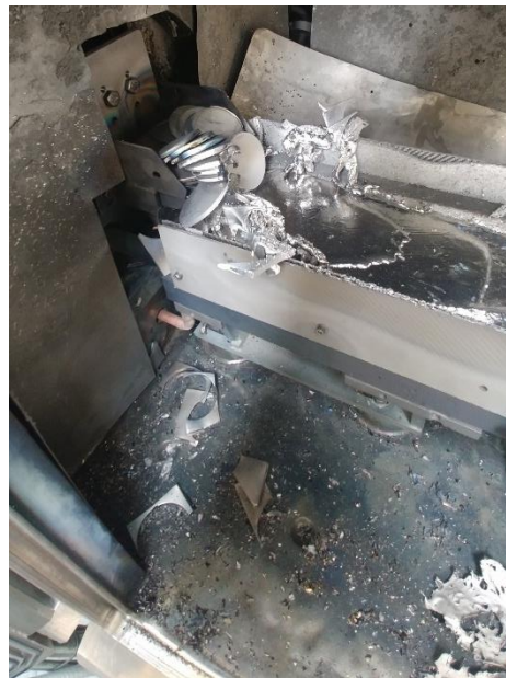
Fig. 4.4. Photographs of the CHM chamber after scrap melting depicting the ingot withdrawal mechanism in the ingot removal position (left) and un-melted scrap and coins built up before the hearth and lying on the chamber floor after falling off the edge (right)
