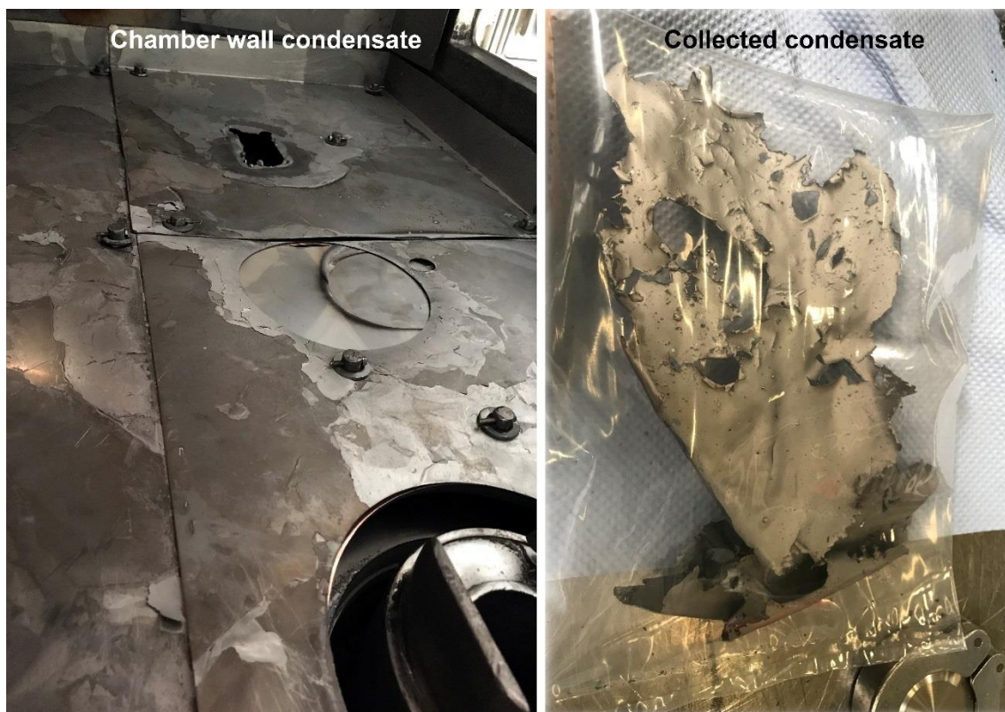
Fig. 3.3. Photographs of condensate from Ti-Nb melting process on the chamber shroud (left) and collected during chamber cleaning (right)
