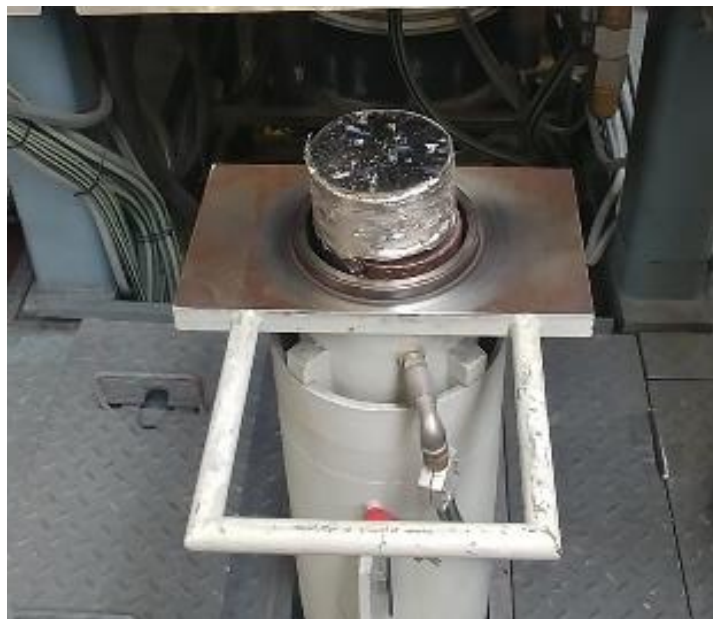
Fig. 4.4. Photographs of the CHM chamber after scrap melting depicting the ingot withdrawal mechanism in the ingot removal position (left) and un-melted scrap and coins built up before the hearth and lying on the chamber floor after falling off the edge (right)
