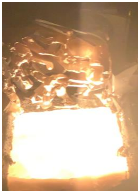
Fig. 4.3. Photographs of scrap melting in the ALD CHM furnace
