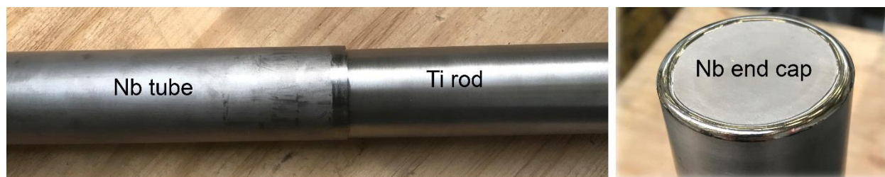
Fig. 2.1. Photograph of Ti rods and Nb tubes from Admat
