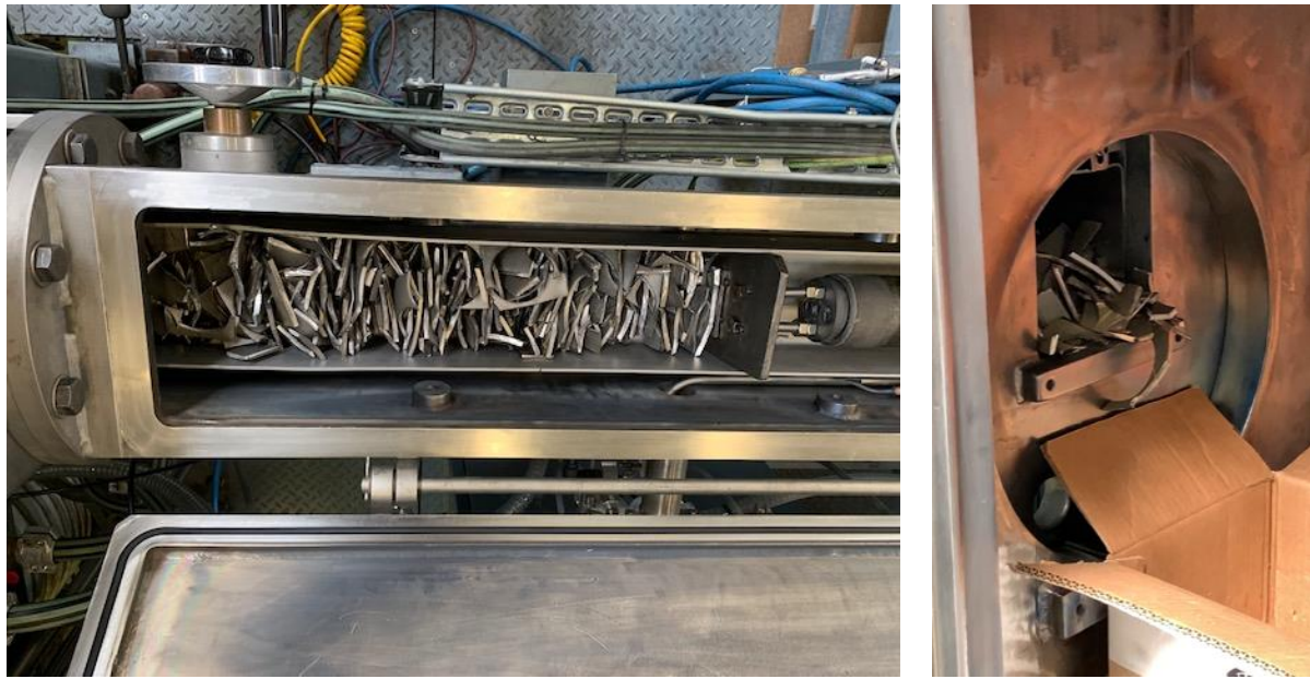
Fig. 4.1. Photographs of titanium scrap loaded into the bar feeder chamber (left) and delivery into a box (right)
