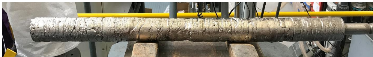
Fig. 3.5. Ingot 2 outer surface showing irregularities due to ingot withdrawal speed
