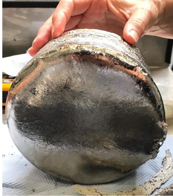
Fig. 4.5. Photograph of ingot produced from recycled scrap
