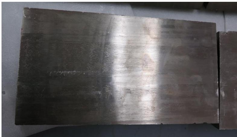
Fig. 3.6. Photograph of the top half of Ingot 1, measuring 10.5" x 5.75" x 3" after cross-sectioning via wet saw
