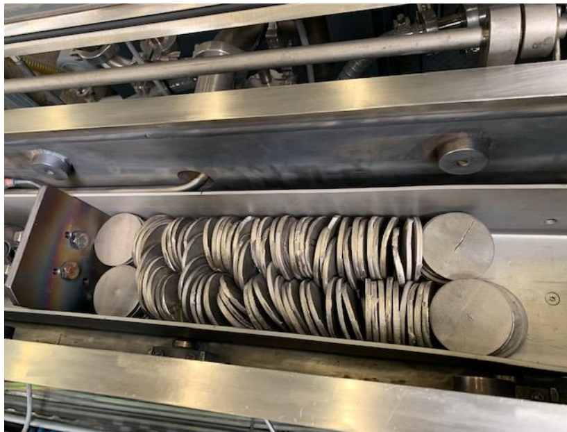
Fig. 4.2. Bar feeder loaded with coin material
