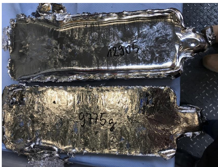
Fig. 3.2. Photographs of Ti hearth from Nb tube filling (bottom) and Ti-Nb hearth from alloying (top)
