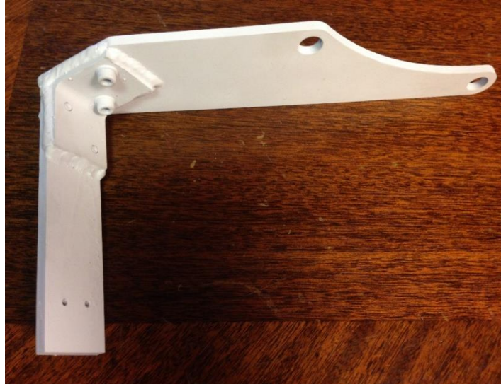
Bracket: 1/4 inch steel welded, bolted for initial alignment.
