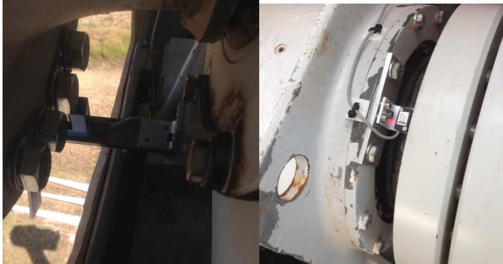
Figure 4. left) Image of OSPR installed on mounting bracket, right) Second low speed shaft overspeed sensor (OSPS).
