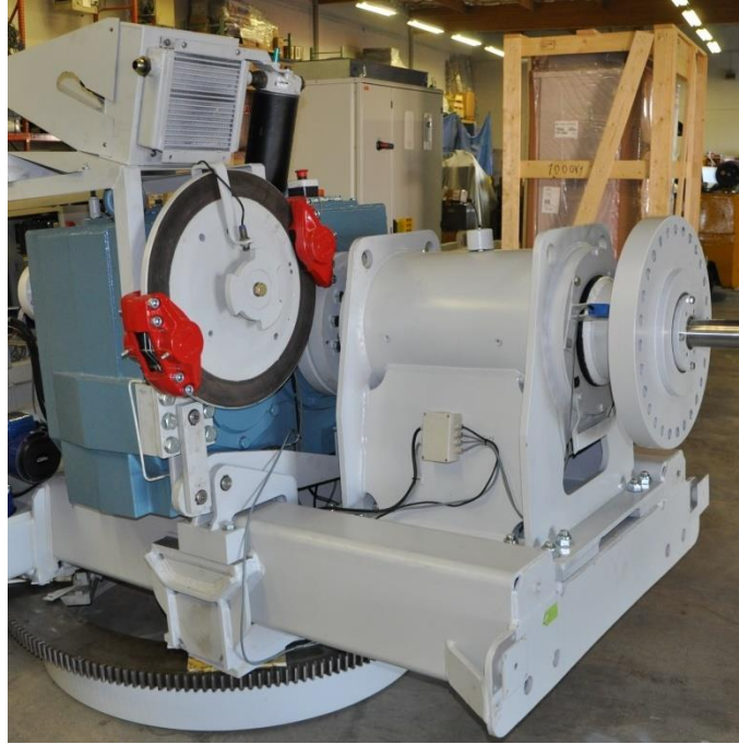
Figure 14. SWiFT Nacelle during construction showing high speed shaft brake mounted to gear box housing.
