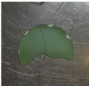
Figure 2-86 Cracked Substrate, RSDT Deposition #1062 Trial 1
