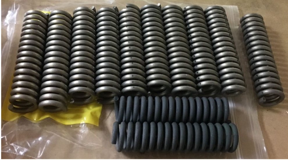
Figure 3-14 Springs – as wound (top) and heat treated (bottom)
