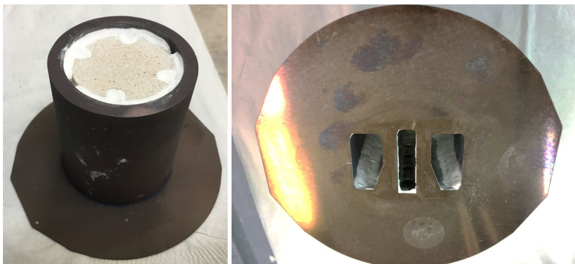
Figure 3-21 Inner fuel manifold seal testing jig
