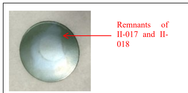
Figure 2-111 #1186-2 before being deposited in #1996. The small LSCF remnants from II-017 and II-018 occupy a circular area indicated by the red arrow.
