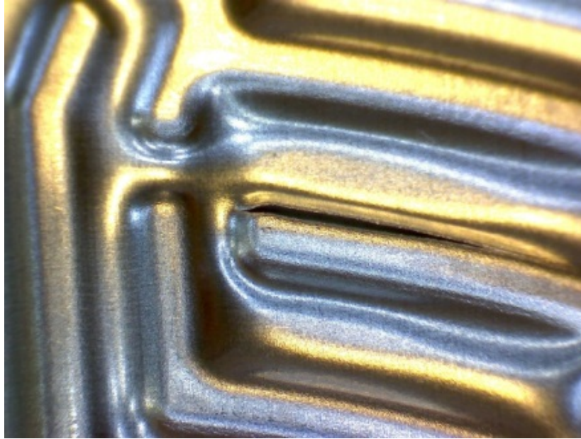
Figure 3-58 Cracks in First Design Revision
