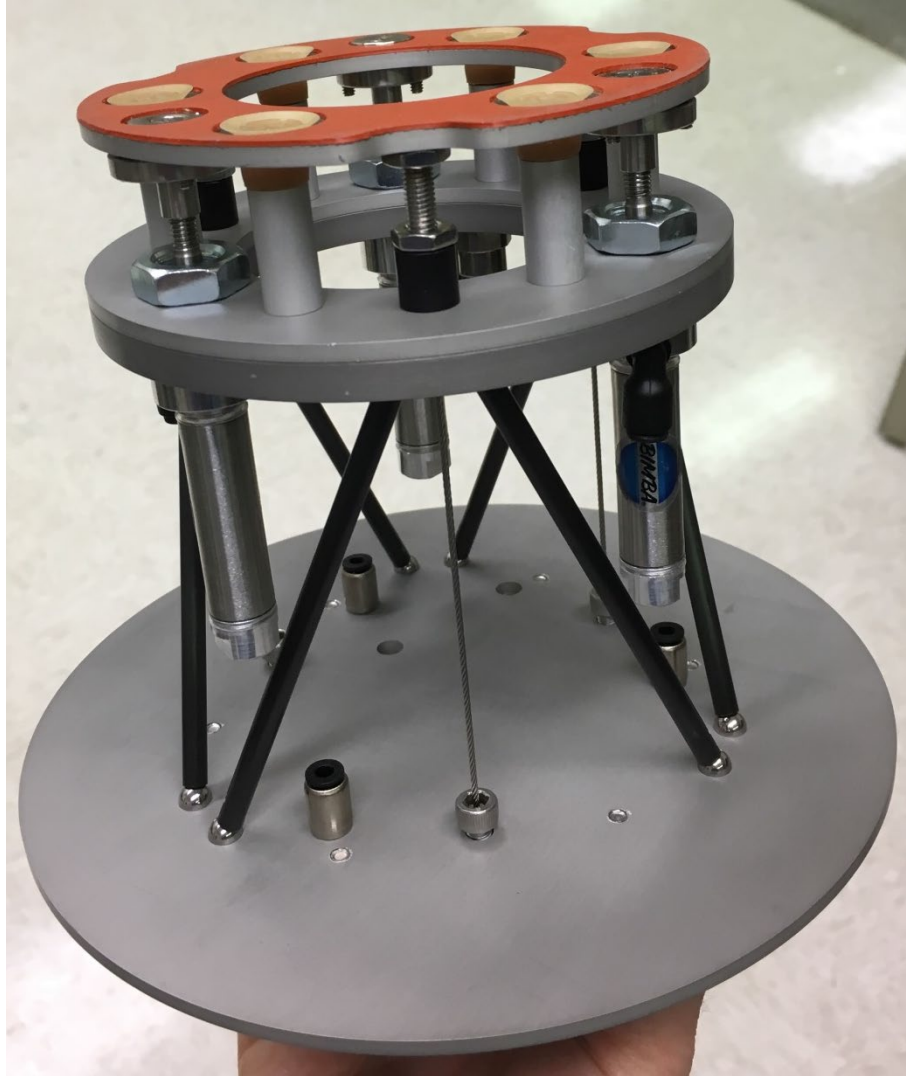
Figure 3-85 Robot end effector
