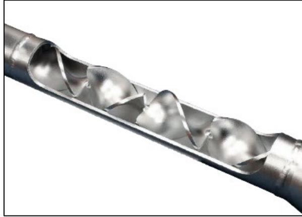
Figure 2-58 Static Mixer (Cut Away View) [Ref. 5]. Each Blade Segment Reverses the Flow from Right to Left Along the Flow Axis
