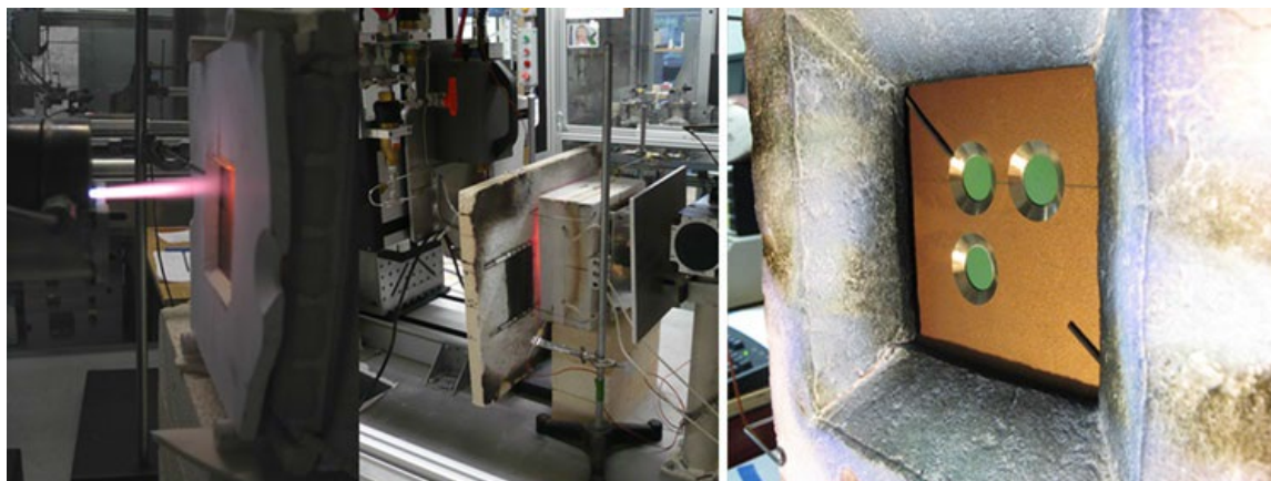
Figure 2-118 RSDT deposition with furnace, from left to right, side view of deposition, back view of furnace, metal mask holding substrate.
