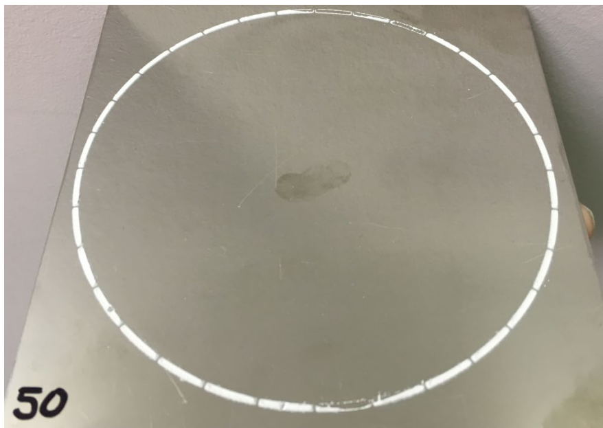
Figure 3-76 As dispensed seal (missing areas due to handling, not printing)
