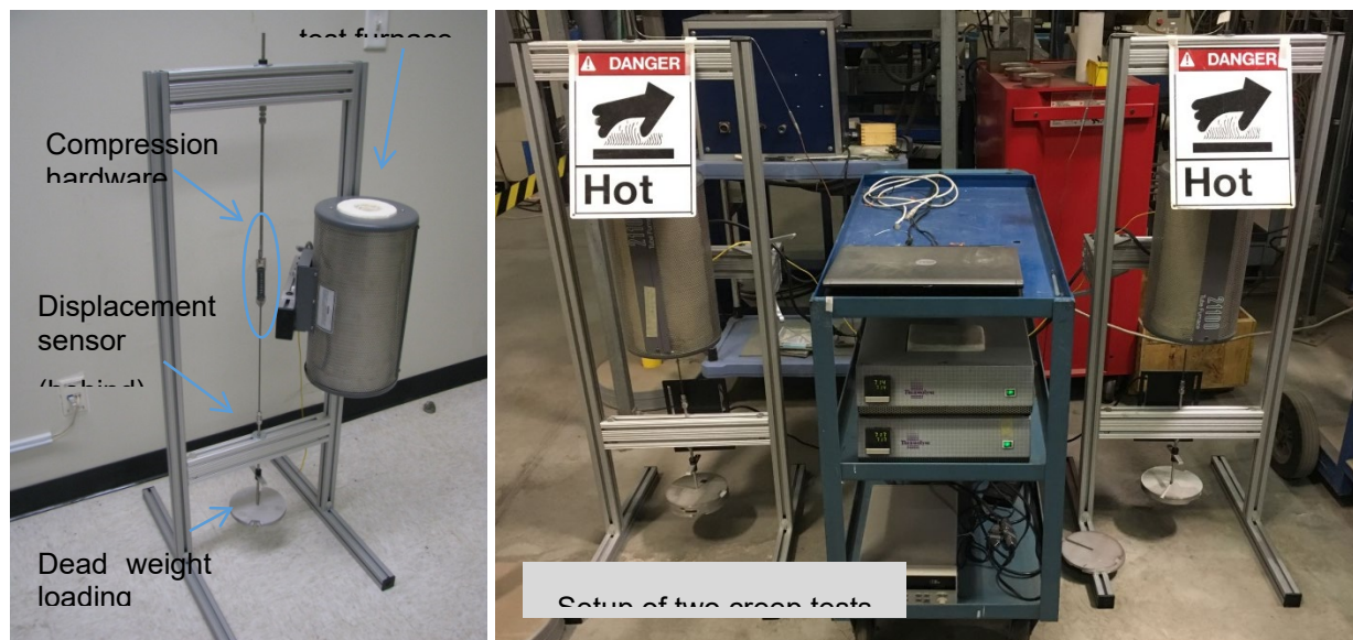
Figure 3-8 Creep Tester Setup for Compression Hardware Testing
