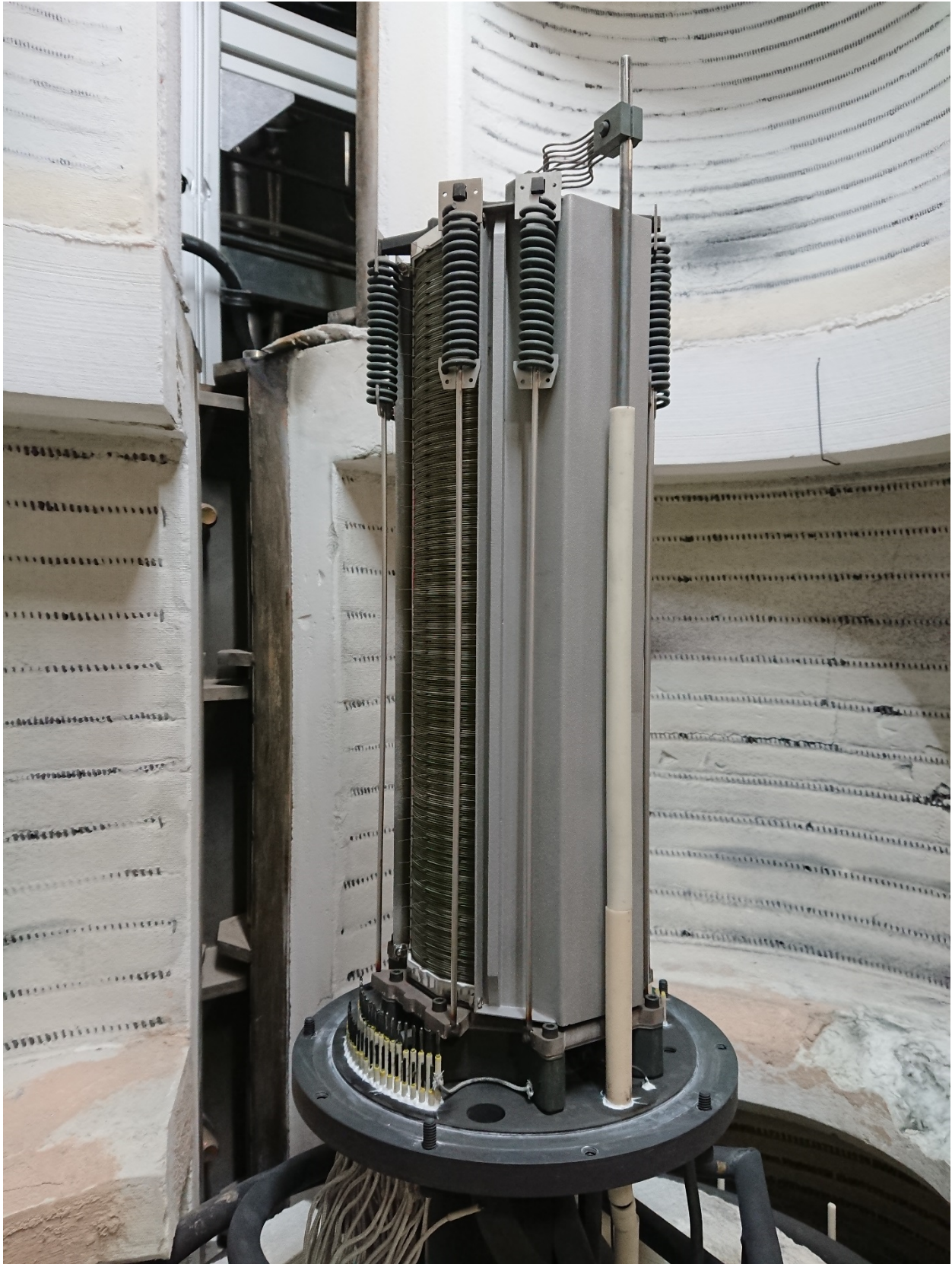
Figure 4-56 First full height CSA stack installed into test stand
