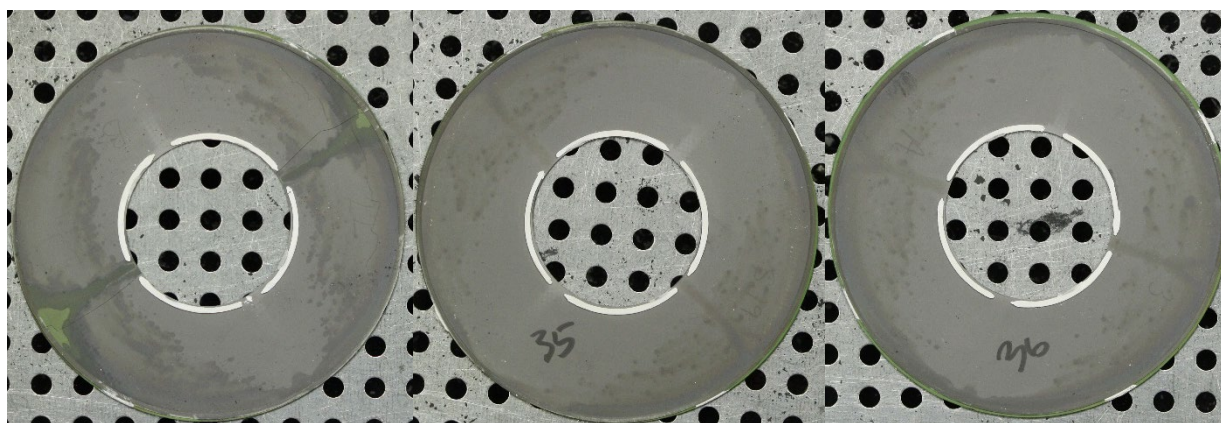
Figure 4-46 GT060248-0011 Cells 34-36 oxidation patterns
