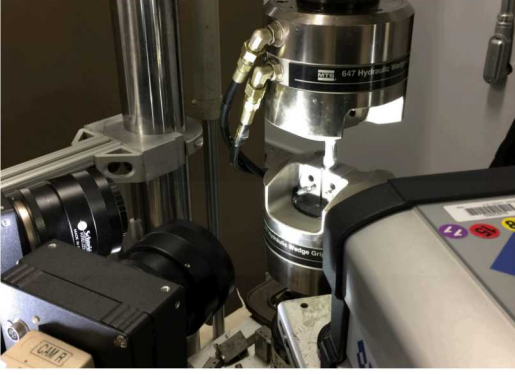
Figure 4: Test setup for Solid_Torsion_3.
