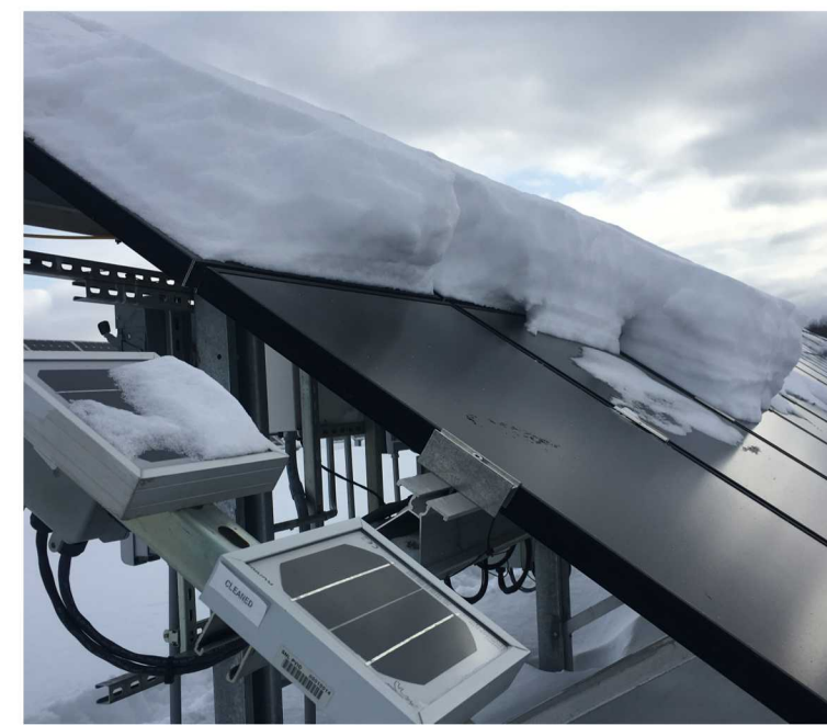
Figure 4. Differential snow shedding across monolithic CIGS modules creates electrical stress
