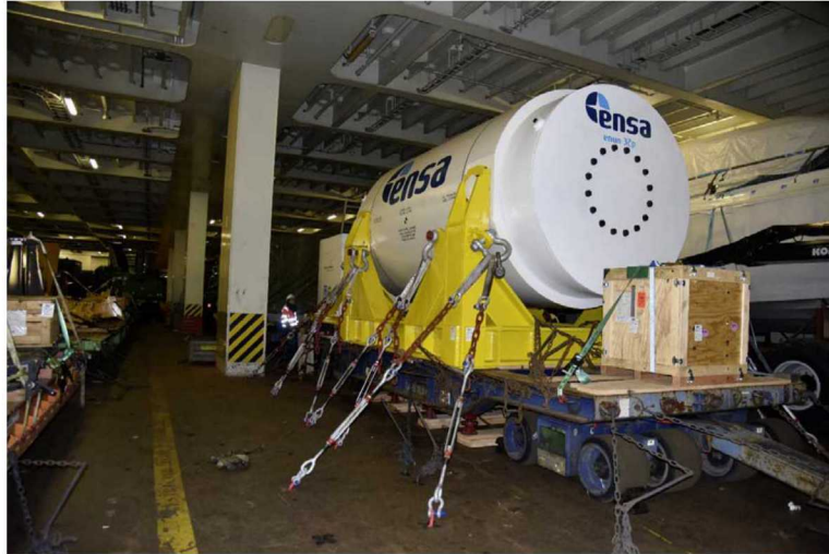
FIG. 7. Cask lashed to the interior deck of the ocean ship "Tarago."
