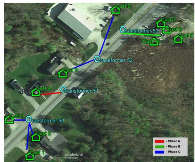
Figure 11. Spectral clustering predicted phase connections of 10 customers connected through 4 transformers as shown, validated with Google Street View.
