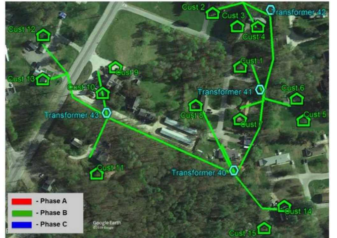
Figure 7 - Topology validation showing an incorrectly labeled lateral
