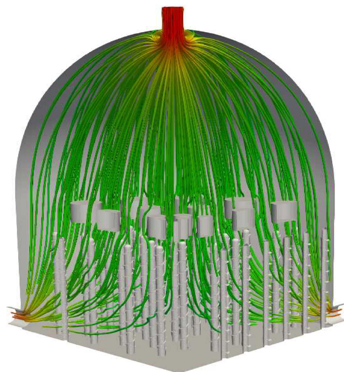
CFD simulation of the sCO 2 -Heat Pipe Interface: velocity streamlines.
