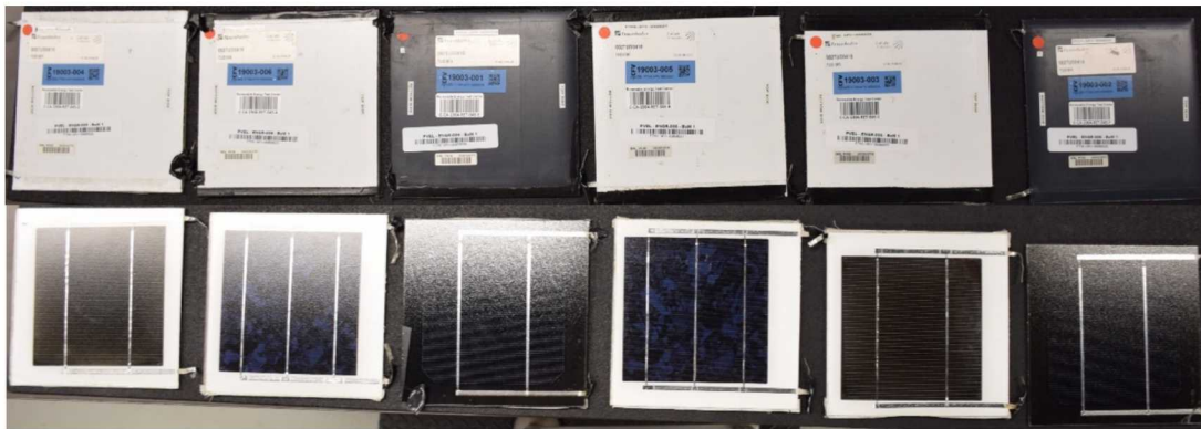
Figure 2-1 Six Laminated Cells with Exposed Tabbing Ribbon (Top – Back, Bottom – Front)
