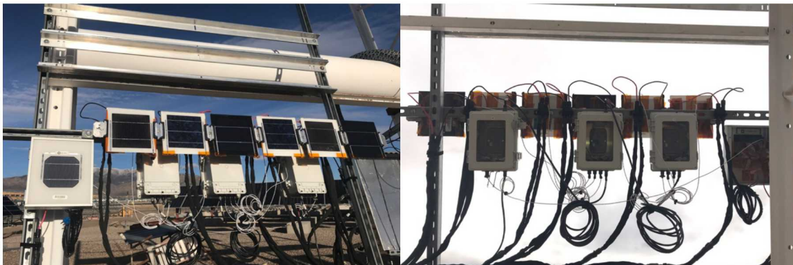
Figure 2-2. Six Laminated Cells Mounted on Sandia's Two-Axis Solar Tracker
