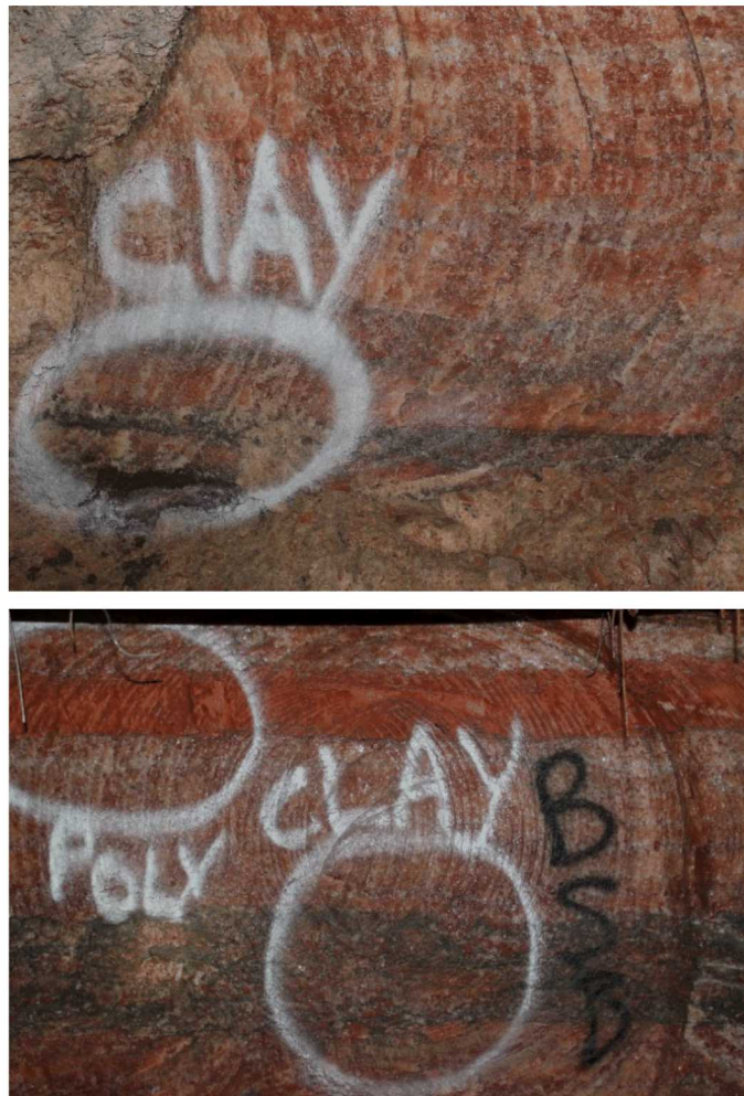
Fig. 4. Exposed Clay Seam (Top) and Halite/Polyhalite Contact (Bottom) for Test Core Collection (regions in photos are approximately 6 feet wide).
