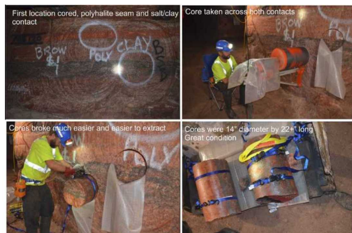
Fig. 5. Core extraction from side wall of drift.
