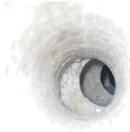
Fig. 2. Example of interface sliding in a borehole at WIPP.
