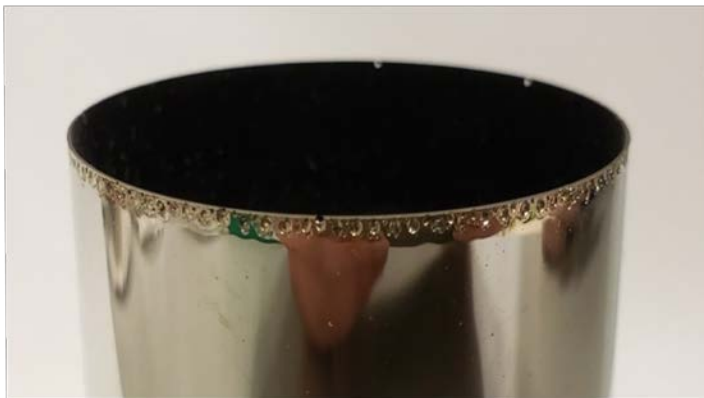
Figure 5. End of optic shows pits which effects final figure of optic. This was result of not enough surfactant in bath.
