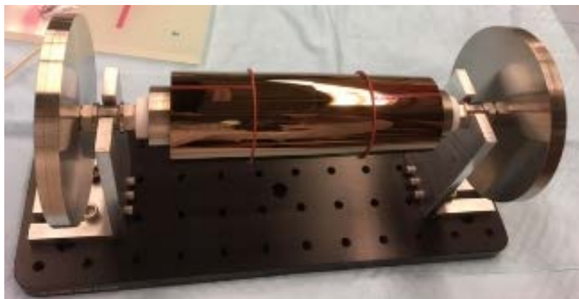
Figure 1. SANZ1b mandrel shown on inspection station fixture. Mandrel is 139 mm long with optic length 60.97 mm. Optic is central part with end cap on either side. End caps are necessary to provide uniform fields during fabrication but are not part of the final optic.
