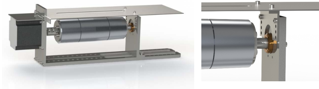
Figure 10. Left: Engineering design showing modified mandrel fixture housing with mandrel slit plate. Right: Detail design of bushing and end plate to support mandrel while rotating.
