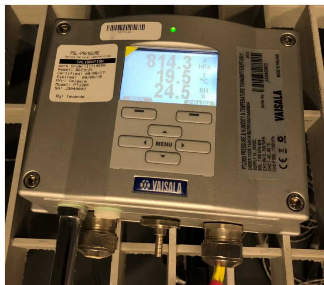
Figure 8 Vaisala PTU300 Temperature, Pressure, and RH within Infrasound Chamber
