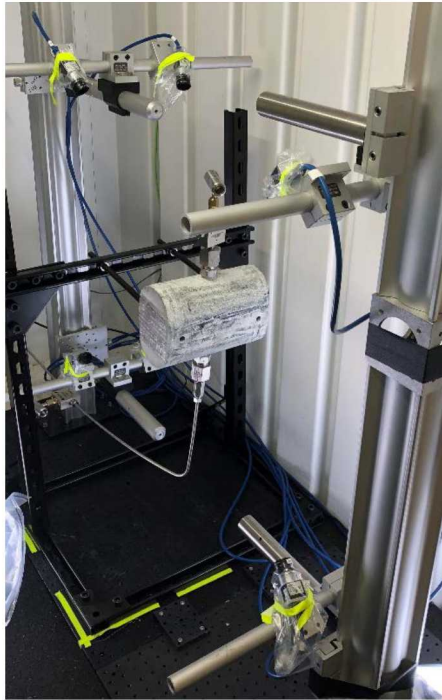
Figure 9, Experimental setup with TA in center and DIC cameras surrounding
