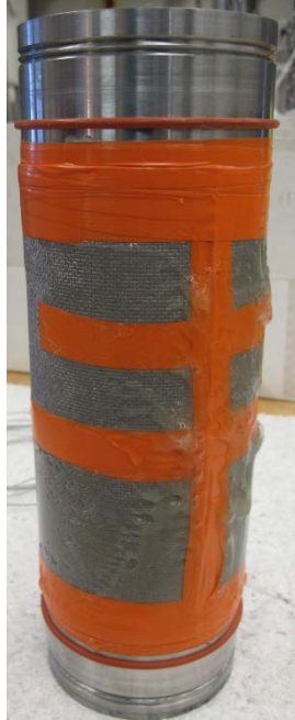
Figure 9. Westerly granite fracture specimen assembly
