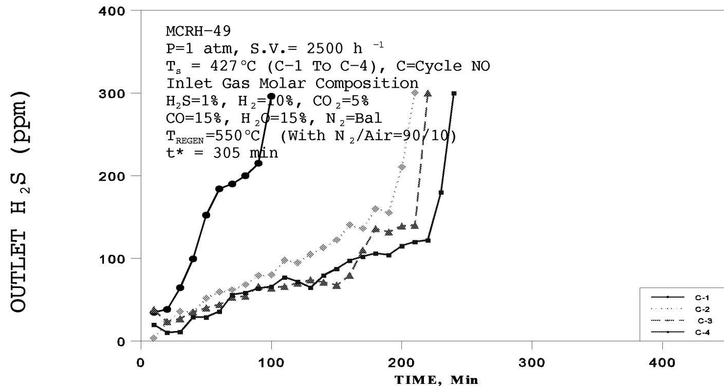
Figure 8.  $\text{H}_2\text{S}$  Breakthrough Curves in Successive Sulfidation Cycles of Sorbent MCRH-49
