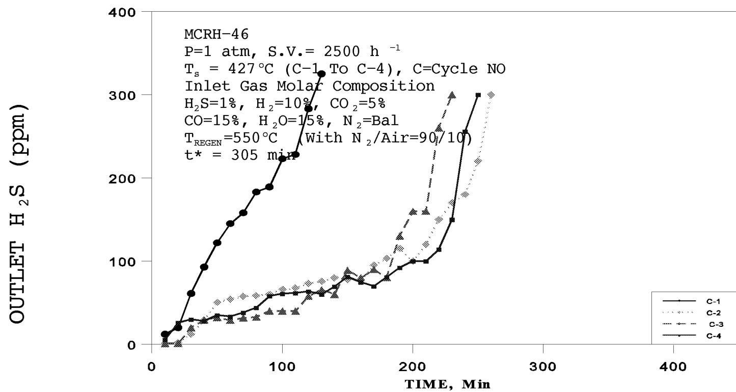
Figure 6.  $\text{H}_2\text{S}$  Breakthrough Curves in Successive Sulfidation Cycles of Sorbent MCRH-46
