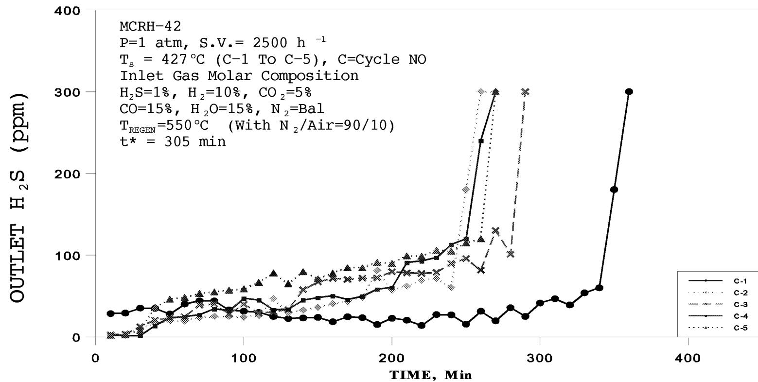
Figure 2.  $\text{H}_2\text{S}$  Breakthrough Curves in Successive Sulfidation Cycles of Sorbent MCRH-42
