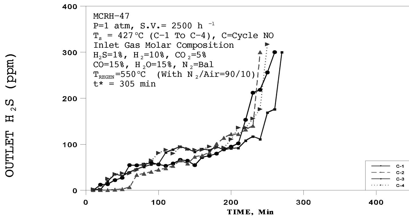
Figure 7.  $\text{H}_2\text{S}$  Breakthrough Curves in Successive Sulfidation Cycles of Sorbent MCRH-47
