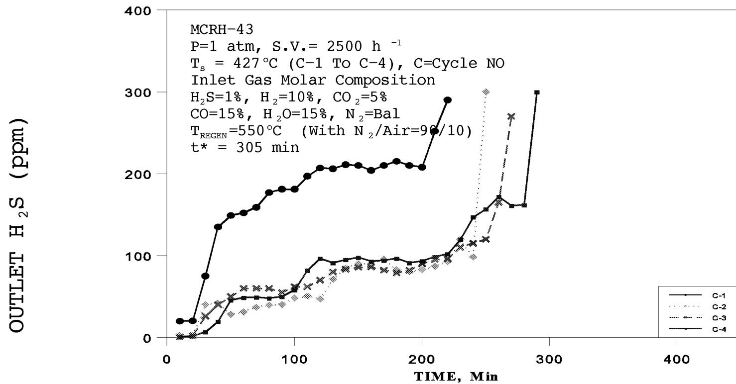
Figure 3.  $\text{H}_2\text{S}$  Breakthrough Curves in Successive Sulfidation Cycles of Sorbent MCRH-43
