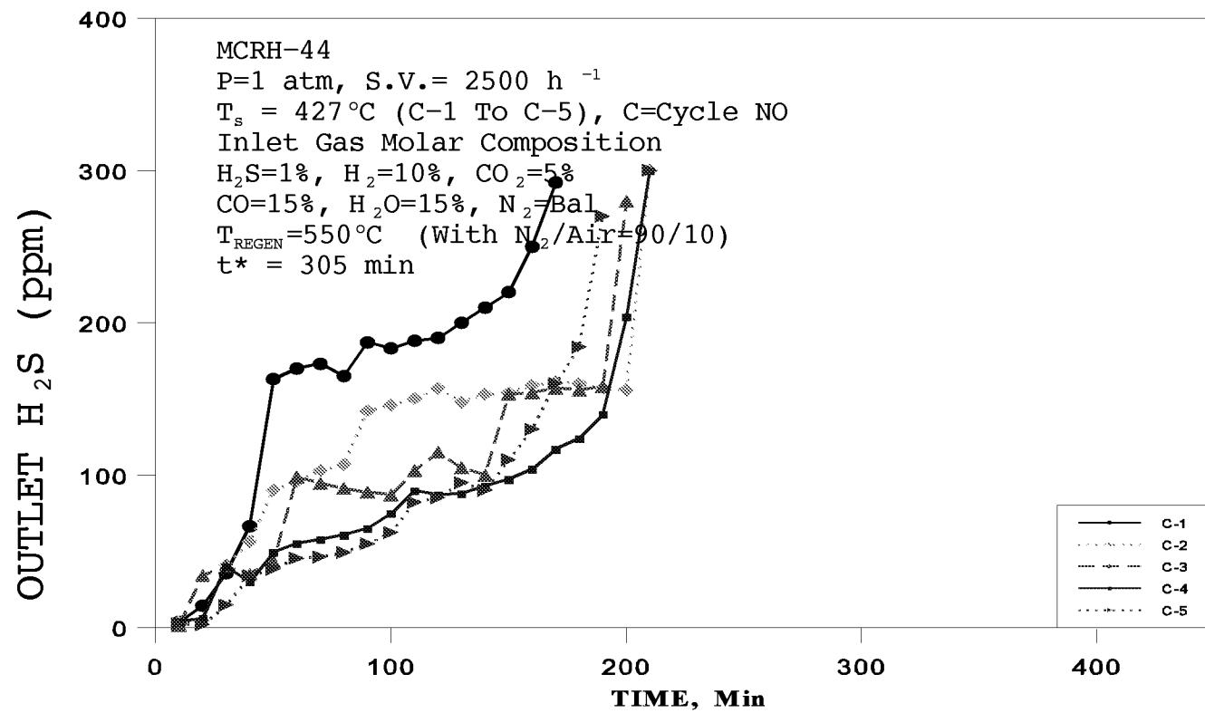
Figure 4. H<sub>2</sub>S Breakthrough Curves in Successive Sulfidation Cycles of Sorbent MCRH-44
