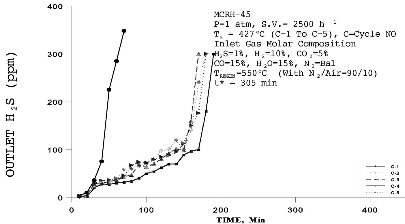
Figure 5.  $\text{H}_2\text{S}$  Breakthrough Curves in Successive Sulfidation Cycles of Sorbent MCRH-45
