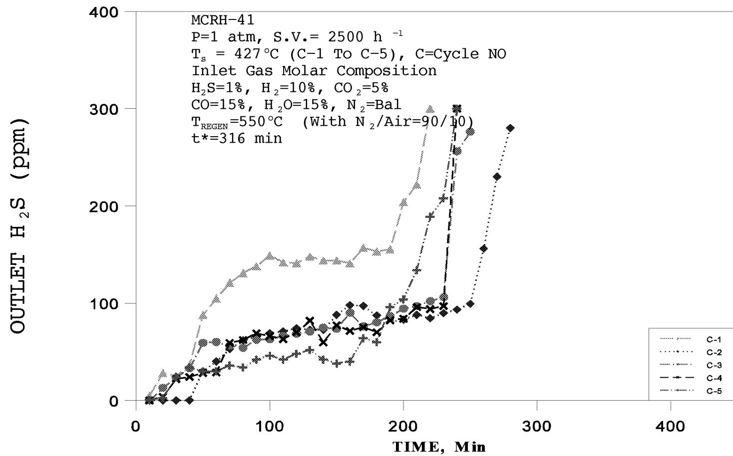
Figure 1.  $\text{H}_2\text{S}$  Breakthrough Curves in Successive Sulfidation Cycles of Sorbent MCRH-41
