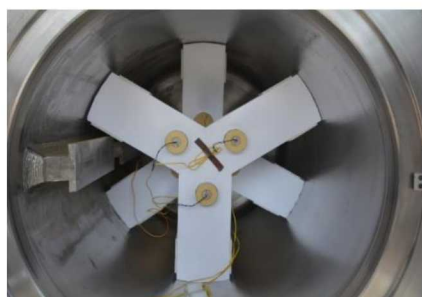
Figure 3: Six 1.5 lb C-4 charges (11.25 lb TNT equivalency) arranged in the V28 vessel.
