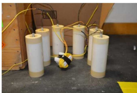
Figure 2: Individual charges packed into plastic bottles—detonator adapter shown at center.
