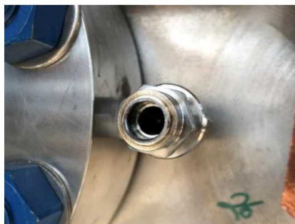
Figure 20: Failed fitting as found on feedthrough flange post-shot
