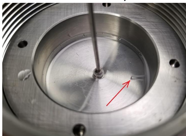
Figure 7. Pinhole the bellows top plate.
