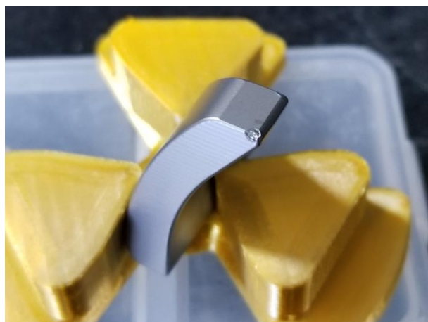
Figure 15. Damage / indentation at the tip of one of the levers resulting from touching the second lever during pressurization.
