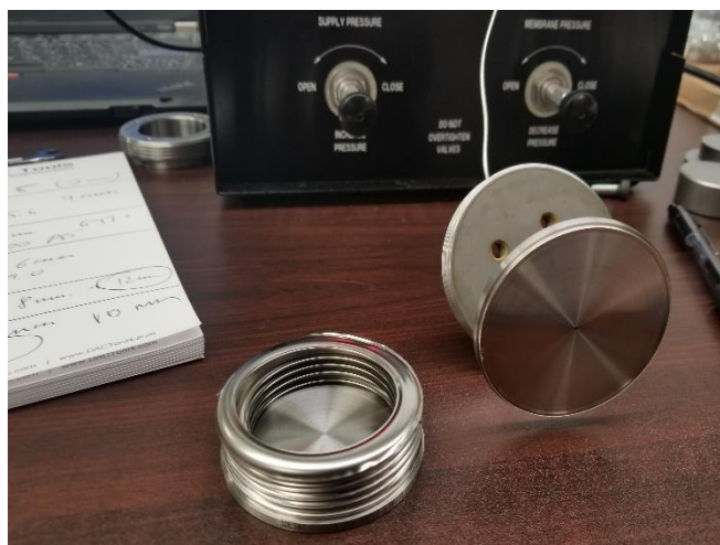
Figure 12. Broken bellows – the bellows ruptured at \sim 10 mm displacement at 2500 PSI.
