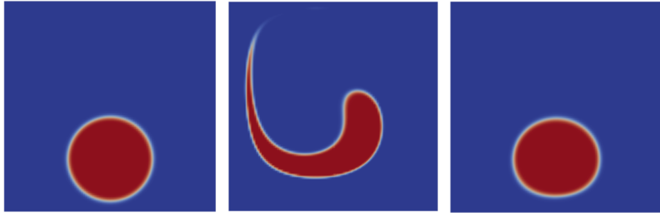
Figure 4.11. Pseudo-VOF field reconstructed from CVFEM level set result at 0, 1000, and 2000 time steps
