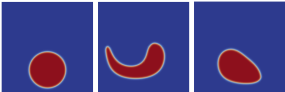
Figure 4.13. Pseudo-VOF field reconstructed from CVFEM redistanced level set result at 0, 1000, and 2000 time steps
