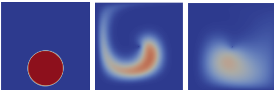
Figure 4.15. VOF with MUSCL+SuperBee advection at 0, 1000, and 2000 time steps
