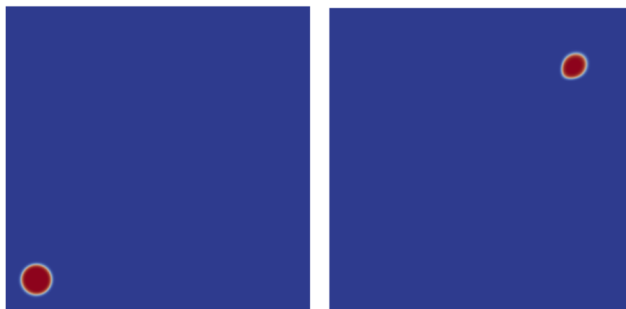
Figure 4.3. Pseudo-VOF field reconstructed from CVFEM level set advection at time steps 0 and 800
