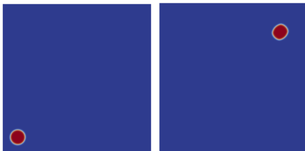
Figure 4.4. Pseudo-VOF field reconstructed from redistanced CVFEM level set at steps 0 and 800
