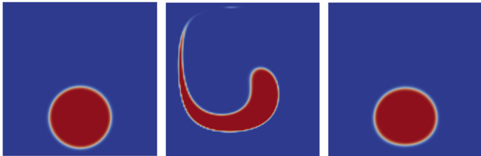
Figure 4.12. Pseudo-VOF field reconstructed from GFEM level set result at 0, 1000, and 2000 time steps
