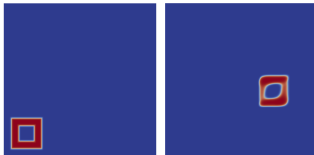
Figure 4.7. Pseudo-VOF field reconstructed from the CVFEM level set solution at time steps 0 and 500
