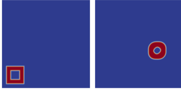
Figure 4.8. Pseudo-VOF field reconstructed from the re-distanced CVFEM level set at time steps 0 and 500
