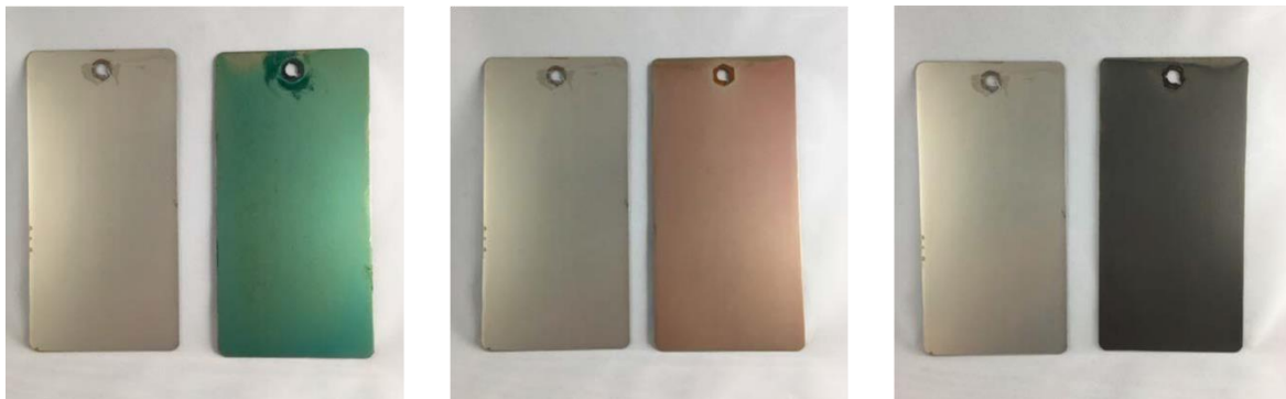
Figure 11. Examples of dyed steel surfaces with anodizing dyes. Left image shows the original panel and the right image shows the subsequently dyed panel in green, red and black.
