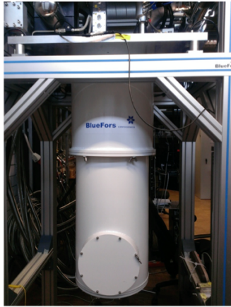
Figure 1 (left): LLNL dilution refrigerator for MMC detector operation at temperatures down to <10 mK. The MMC detector array is held behind the round cold finger at the bottom of the cryostat. The center of the flange is thinned out so that the MMC can detect gamma-rays from external sources. Figure 2 (left): The cooldown from room temperature to <10 mK is automated, does not require cryogenic liquids, and takes about \sim 1 day.
