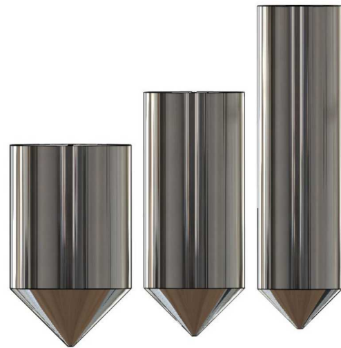
Figure 6: Hopper designs with identical volume configured with increasing height/diameter ratios.
