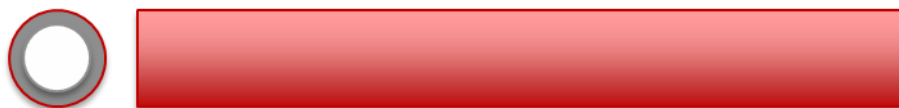
Figure 1. Geometry of open tube with inner surface of tube coated with metal hydride. Tube is typically much longer vs. its diameter than illustrated here.
