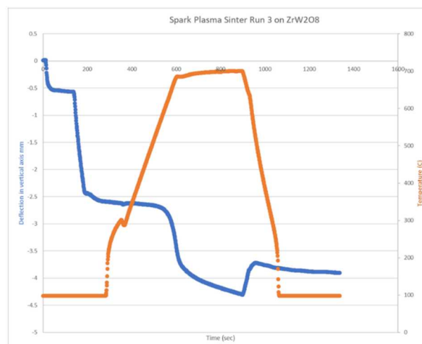
Fig. 1. Sintering procedure for \text{ZrW}_2\text{O}_8 . Maximum applied temperature was 700^\circ\text{C} (orange line), maximum pressure was 60 MPa, both held for 5 minutes. The blue line denotes the ram position.
