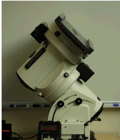
Astro-Physics 1600GTO • German Equatorial Mount • Load Capacity 210 Lbs.
