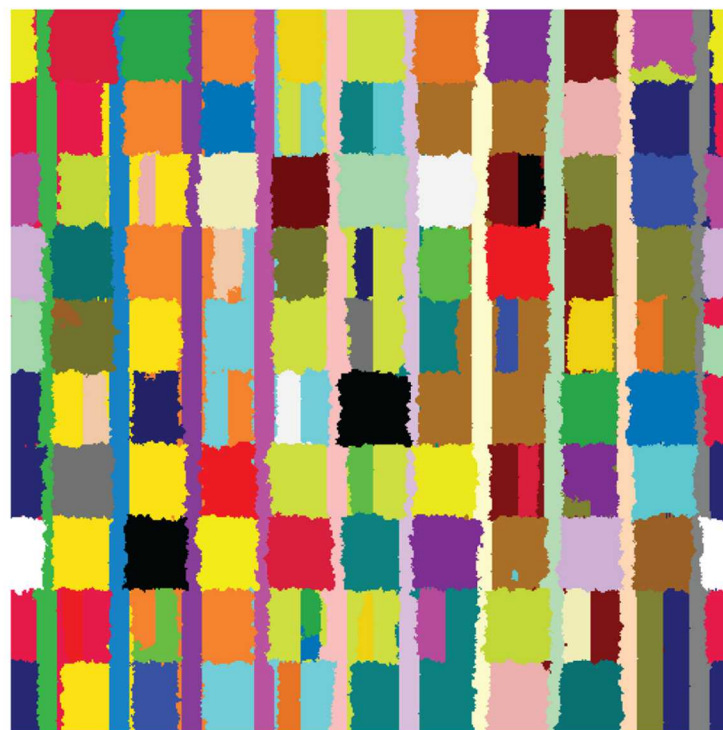
(b) after annealing at 6 K/min. to 1300 K
