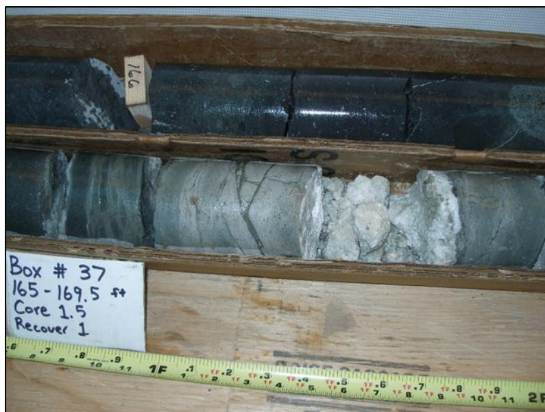
Figure 19: Example of core from AK-3 from ~168' showing an apparent flowing fracture.
