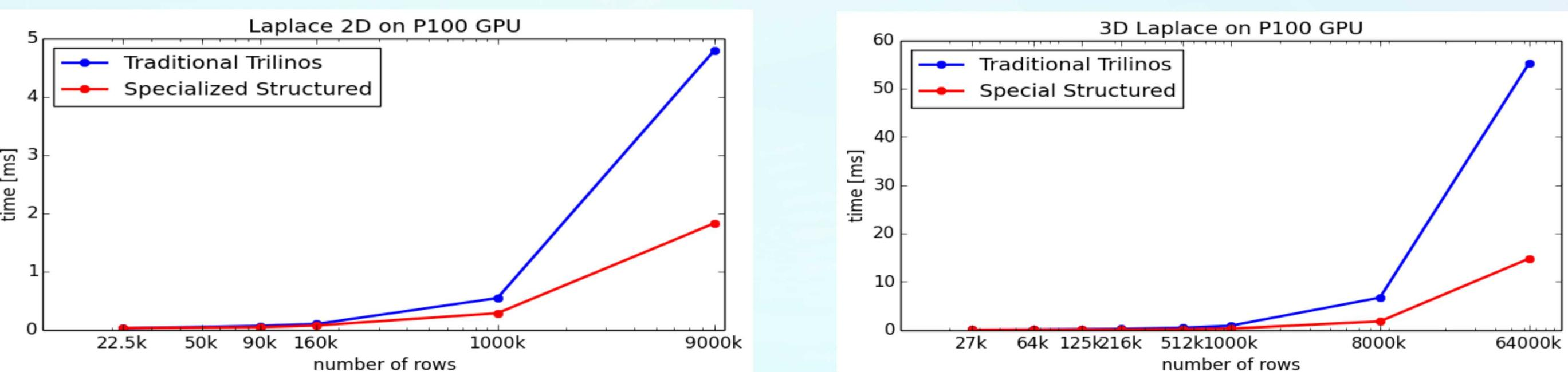
Specialized matrix-matrix multiplies perform RAP triple-matrix products over an order of magnitude faster than standard Trilinos triple-matrix products
