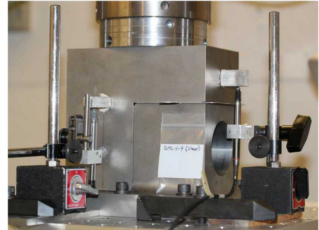
Quasistatic Shear Test Setup
