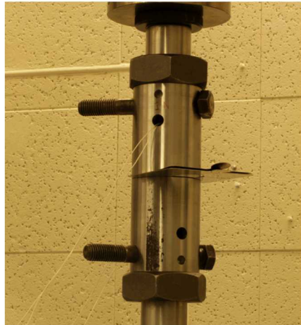
Quasistatic Tension Test Setup
