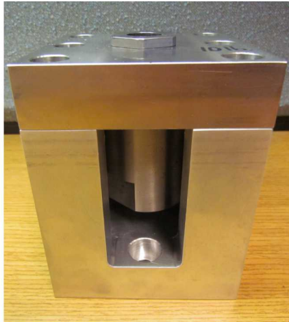
Dynamic Tension Test Setup
