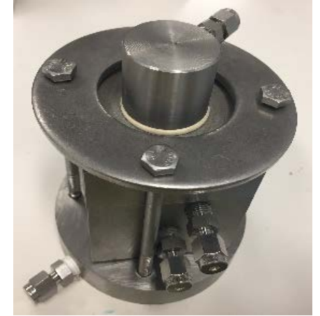
Permeability anisotropy cell: the double-ring method
