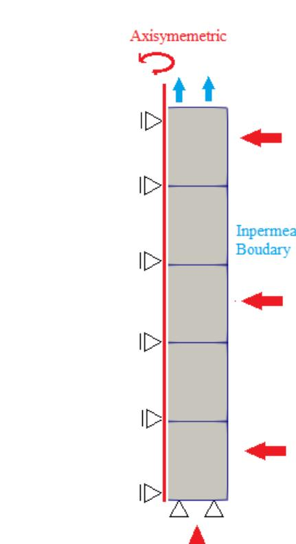
Isotropic consolidation and thermal stimulations modeling for pressure and temperature responses under hydrate dissociation
