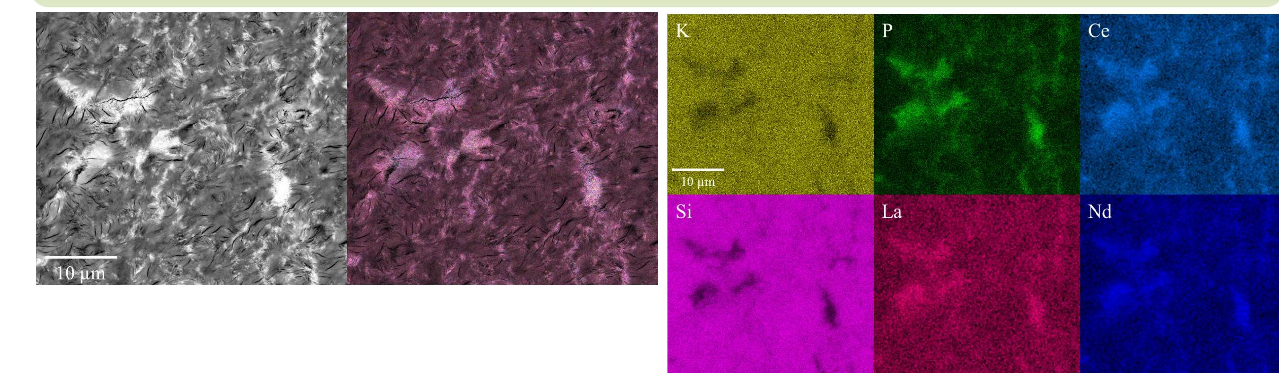
Elemental mapping by EPMA WDS confirms the distribution of the light REEs (La, Ce) in these nano- to micro- scale phosphate minerals (top row of figure below). Qualitative EDS mapping of Er, Tb, and Yb show disseminated occurrences in the glauconitic fabric (bottom row of figure below).
