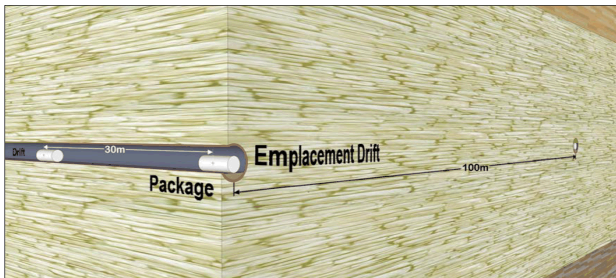
Figure 2-7. In-drift disposal after emplacement and during repository ventilation, prior to installation of backfill then repository closure
