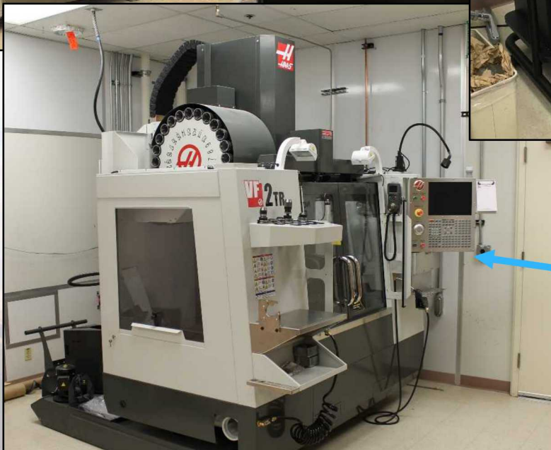
Haas VF2 mill-turn machine will be Modified for Multi-Material hybrid AM, including LENS™
