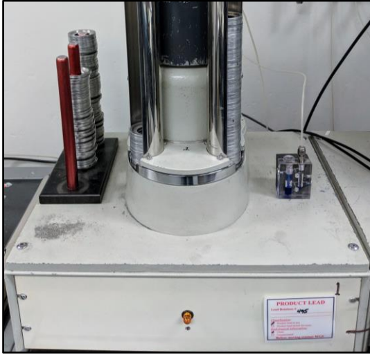
Fig. 1. The legacy 4-Channel beta-particle counting system utilizes proportional gas-flow detectors with automated sample-changers.
