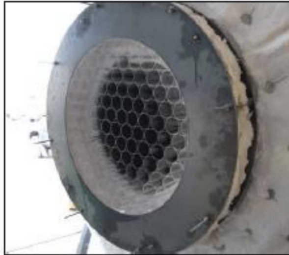
Figure 1 – Quartz-tube window mounted over a 250 kW th cavity receiver aperture
