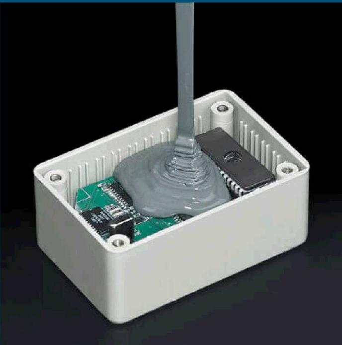
**Potting material design and associated properties are critical to the performance against shock/vibration.**
