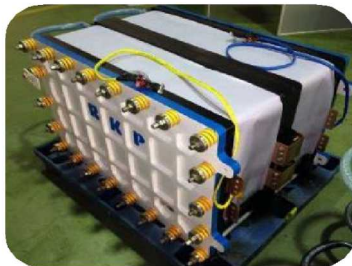
32 KW Stack Rongke Power/UT 120 mA/cm 2 Meter size stack
