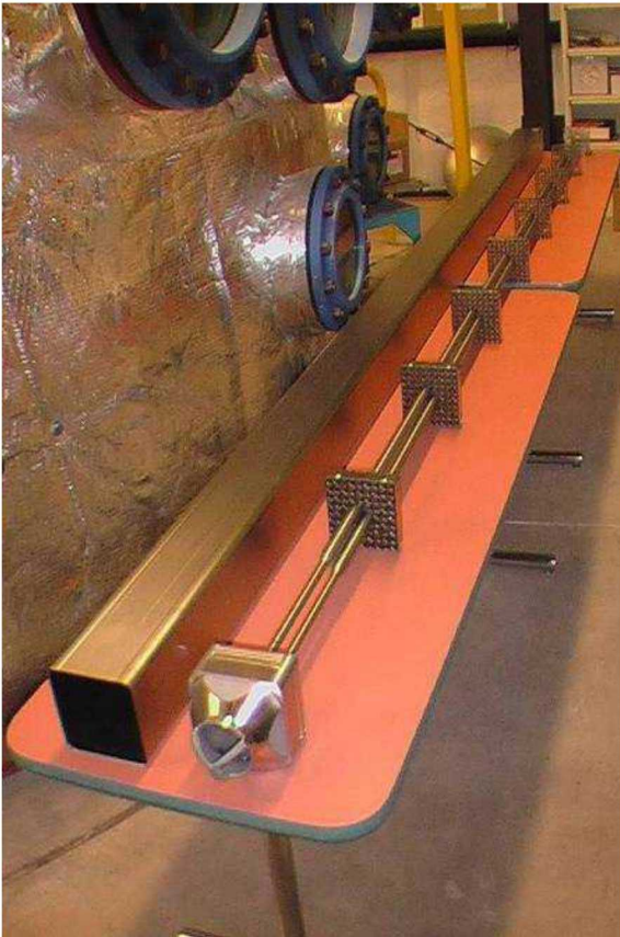
BWR channel, water tubes and spacers
