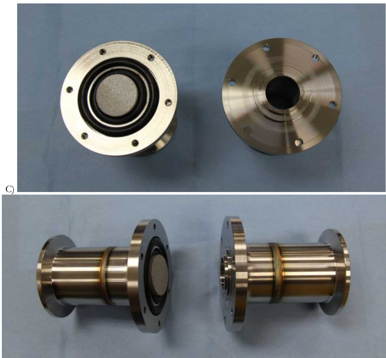
Figure 1. A) shows the experimental system used to characterize the vacuum conductance of porous discs. B) schematically shows the primary components shown in A as well as the gas flow. The components in A and B are in the same locations and orientations. C) Porous sample holder, showing the sealing mechanism with two concentric O-rings.
