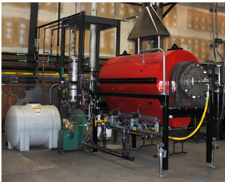
Figure 3: RK-100 rotary kiln for production of CLOU oxygen carrier. The NO 2 absorption tower and caustic circulation system is visible behind the kiln.
